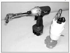
The third iteration of the Makita battery-based power unit, made with PVC pipe and fittings.
