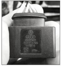
and potted snap-locking connector in common use today. (Heaven help the person charged with its disassembly and repair.) I should not have been surprised to find this VW-Audi logo on our airplane engine's magneto connector, because the Belgian guys behind UL Power began as VW tuners. VWCA
